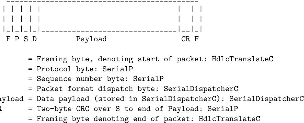
Payload is a contiguous packet that SerialDispatcherC reads in. Note that any data bytes (P - CR) equal to 0x7e or 0x7d will be escaped to 0x7d 0x5e or 0x7d 0x5d accordingly. For example, a platform independent AM packet of type 6, group 0x7d, and length 5 to destination 0xbeef with a payload of 1 2 3 4 5 would look like this:
