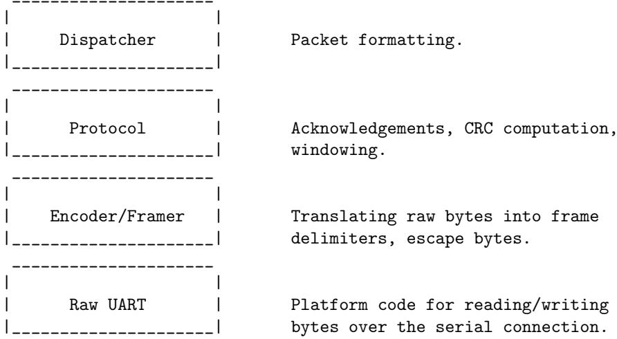
The bottom three provide a byte-level interface: only the Dispatcher provides a packet-level interface. The top three are all platform-independent: only the UART is platform-specific code.
