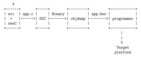
The core TinyOS platforms are centered around GCC, this includes the telos family, mica family and intelmote2. The nesC compiler expects code resembling GCC C-dialect and also outputs code in GCC C-dialect. The current TinyOS platforms are supported by GCC, but for some processor architectures GCC is not available (e.g. Motorola HCS08, Intel MCS51).
