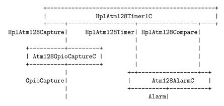
The hardware features is exported using 3 interfaces: HplAtm128Timer, HplAtm128Compare and HplAtm128Capture.
